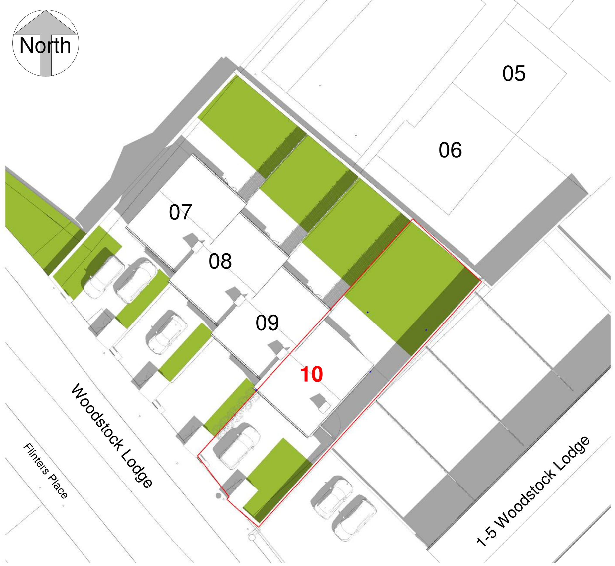
Existing Daylight analysis plan - 20th June at Noon of Site - Summer Solstice 1 : 200
