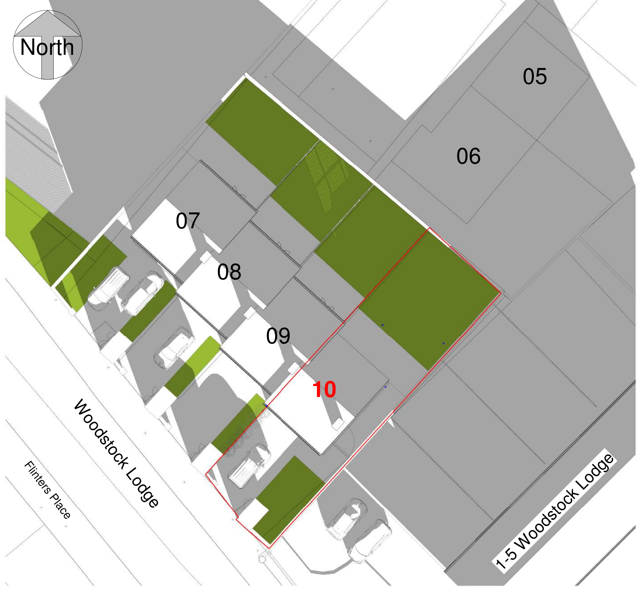
Existing Daylight analysis plan - 21st December at Noon of Site - Winter Solstice 1 : 200
