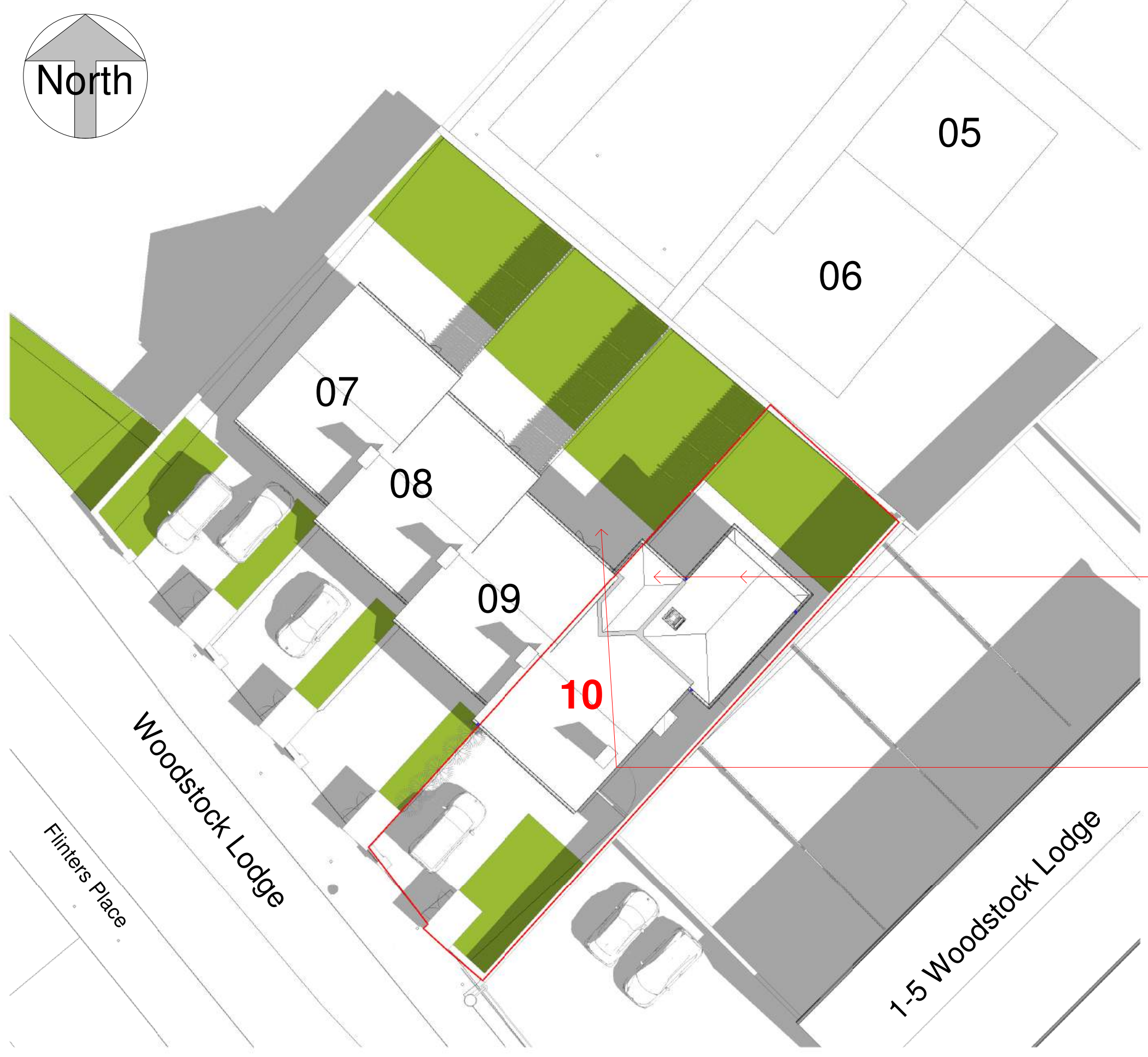
Proposed Daylight analysis plan - 20th June at Noon of Site - Summer Solstice 1 : 200
