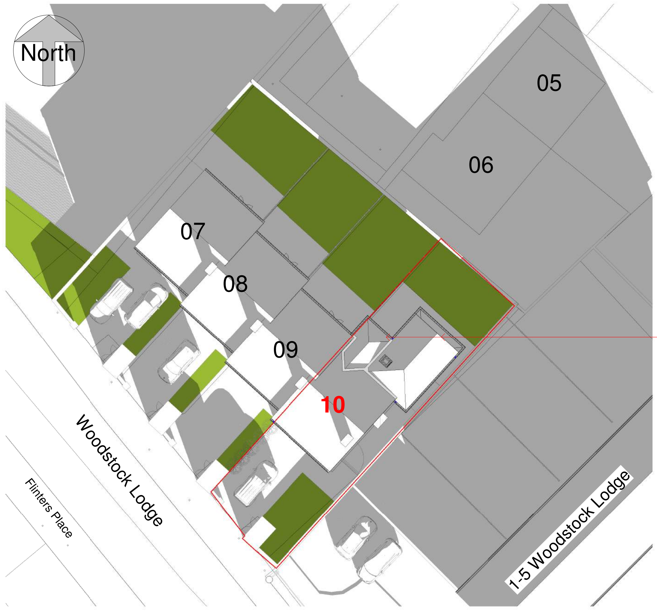
Proposed Daylight analysis plan - 21st December at Noon of Site - Winter Solstice 1 : 200
